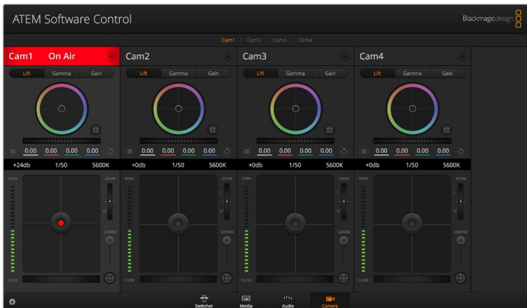
Camera control lets you control Blackmagic Pocket Cinema Camera 4K and 6K with ATEM Mini
