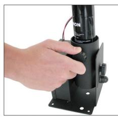
Secure the electric cannon with a screw nut which is situated on the side of the holder.
