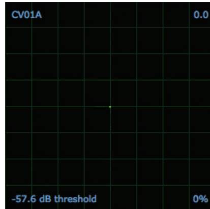
NO SIGNAL - Scratch Live is not receiving any control signal - check your connections.
