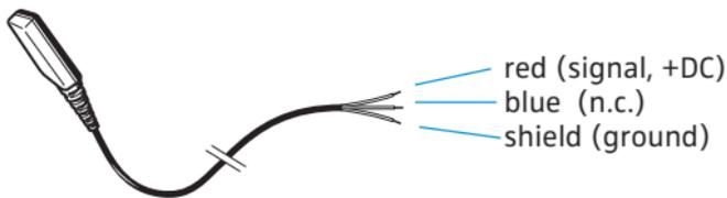
Wiring assignment for adaptation to 3.5 mm jack plug or special connector.
